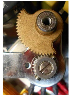
Alignment of the sector and potentiometer gear sets at actuator full CW position. (reference only for Proportional Control units)
