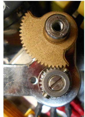
Alignment of the sector and potentiometer gear sets at actuator full CW position. (reference only)
