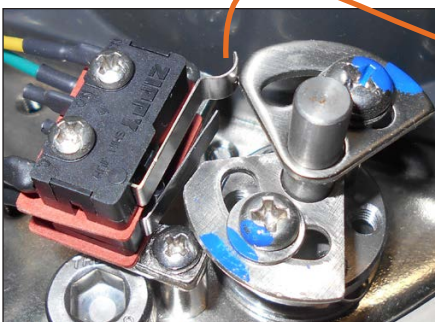
Torque Switch cams shown with the upper cam tripping the upper switch (Actuator was driving CW before this trip)
