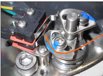
Torque Switch cams shown with the lower cam tripping the lower switch (Actuator was driving CCW before this trip)
