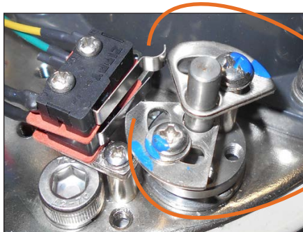
Torque Switch cams and switches are shown in the normal operating position.
