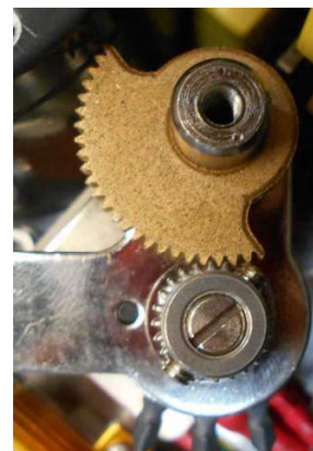
Alignment of the sector and potentiometer gear sets at actuator full CW position. (reference only).
