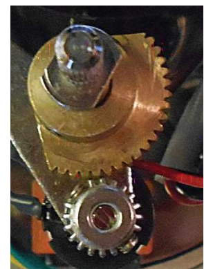
Photo shows the correct alignment of sector gear and pinion gear when the actuator is in its FULL CCW position (CCW cam tripped).
