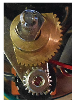
Photo shows the correct alignment of sector gear and pinion gear when the actuator is in its FULL CW position (CW cam tripped).
