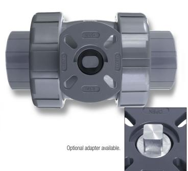
Hayward Flow Control provides a range of mounting options to adapt to our actuators or to your preferred actuator. With the TBH Series ISO top integral flanges, all that is required is just the ISO 5211 coupling and bolting to adapt from the TBH Series stem to Hayward actuators or those actuators with ISO 5211 square drives.
