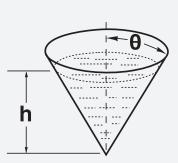
A conical tank with a taper angle of  $25^{\circ}$  is fitted with a 2" diameter short tube type outlet. The area of the outlet is:
