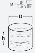
A vertical cylindrical tank 12' in diameter is fitted with a 2" Hayward bulkhead fitting (comparable to a short tube outlet). The area of the outlet is:
